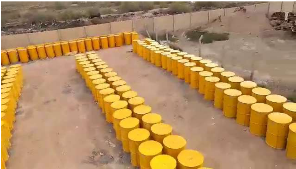
FIGURE 7: Conditioned 450 L LLW drum storage on an external pad in Basra awaiting transfer to Al Tuwaitha
